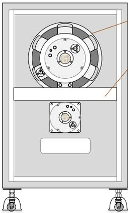
The front portion of the DS701 is supported by 8 pcs. M6 screws, and furthermore the magnetic circuitry is firmly fixed by the inner ledge & aluminium heat-sink, which makes it possible to shut off undesired noises caused by mechanical vibrations that impair sonic quality.
